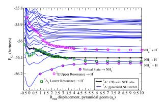
Fig. 1. MR-CIS curves for N-H stretch in  $NH_3^-$ , showing Feshbach resonances from "stabilization" analysis of roots responsible for DEA.
