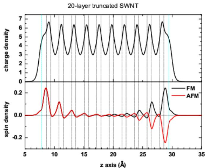
Charge and spin densities for a 20 layer H-terminated truncated SWNT where FM and AFM order are distinguished. Allowance has been made for geometric reconstruction of the tube ends .
