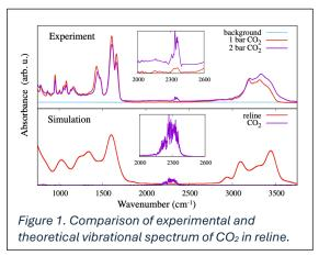
the effect of reline on vibrational spectra of  $CO_2$  and reline. Our simulations indicate that the selective capture of  $CO_2$  from the mixture of  $CO_2$  and  $N_2$  is due to the interplay between attractive electrostatic and charge polarization forces with the opposing entropic effects which shift the energetic balance and makes the  $N_2$  absorption unfavorable in reline.
